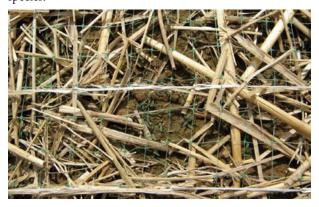
A close-up of a straw erosion blanket is shown here. This and many other types of erosion blankets reduce erosion and increase soil temperature and moisture which favors establishment.
